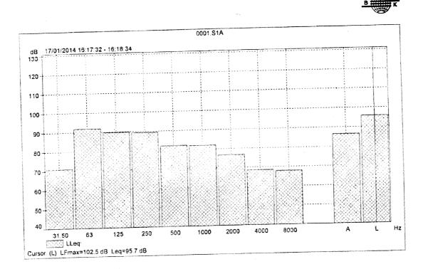
Octave frequency spectrum of sound of music measured at centre of bar, under old archway, at 2 metres from main loudspeakers .
