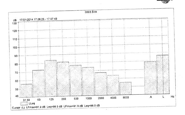
Octave frequency spectrum of sound of music measured at centre of bar, in front of new side street lobby, at 2 metres from main loudspeakers .
